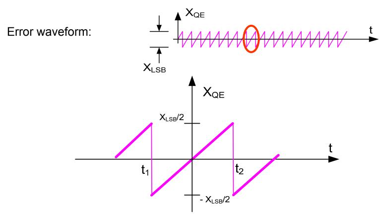
Since  $x_{QE}(t)$  is periodic, the  $X_{QRMS}$  can be obtained by integrating  $x_{QE}^{2}(t)$  over one period
