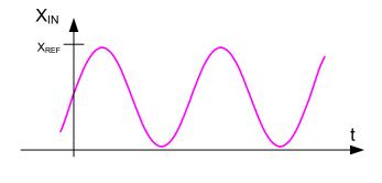
Observe that the RMS value for the sinusoidal signal differs from that of the triangular signal  $X_{SIG-RMS} = \frac{X_{REF}}{\sqrt{12}} = \frac{X_{REF}}{2\sqrt{2}}$
