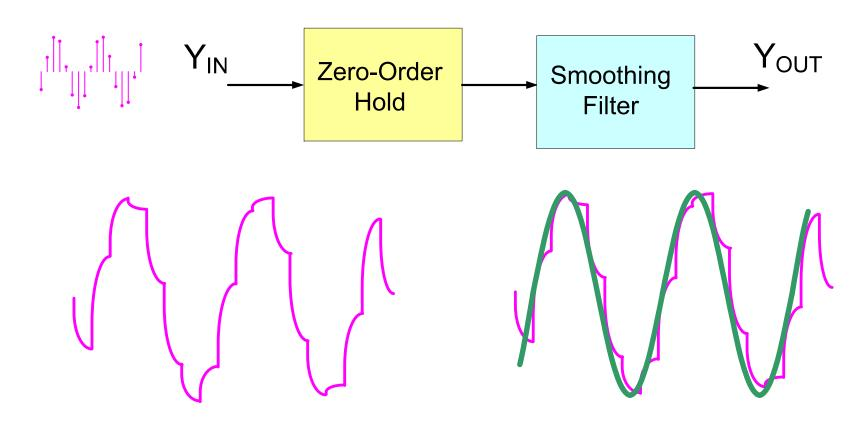
Smoothing filter removes some of the discontinuities in the output of the zero-order hold
