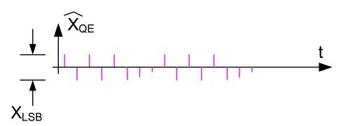
The quantization noise samples of the ADC output are approximately uniformly distributed between in the interval  $[-X_{LSB}/2, X_{LSB}/2]$
